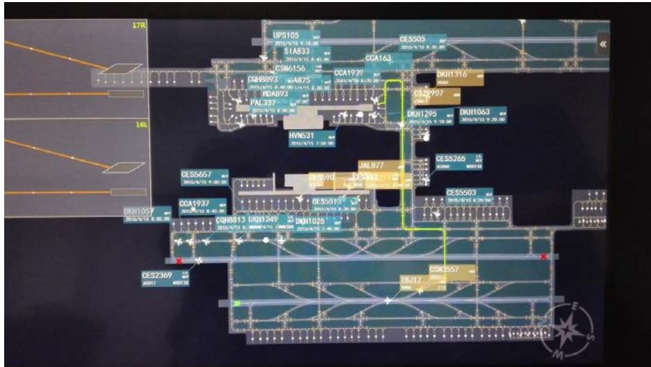
ASMS system interface (the green line is the route planning for an aircraft)
